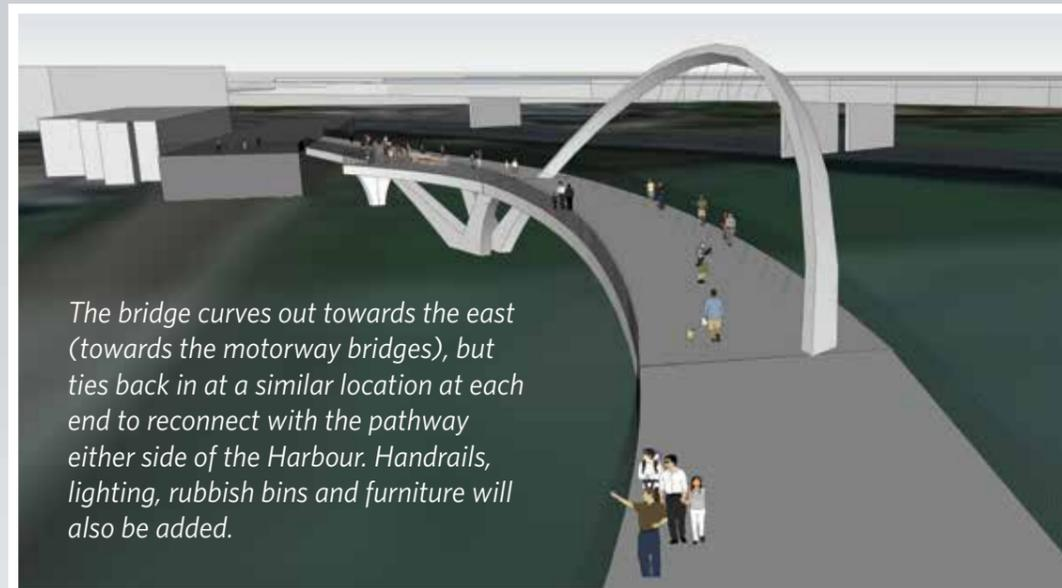
The bridge curves out towards the east (towards the motorway bridges), but ties back in at a similar location at each end to reconnect with the pathway either side of the Harbour. Handrails, lighting, rubbish bins and furniture will also be added.
