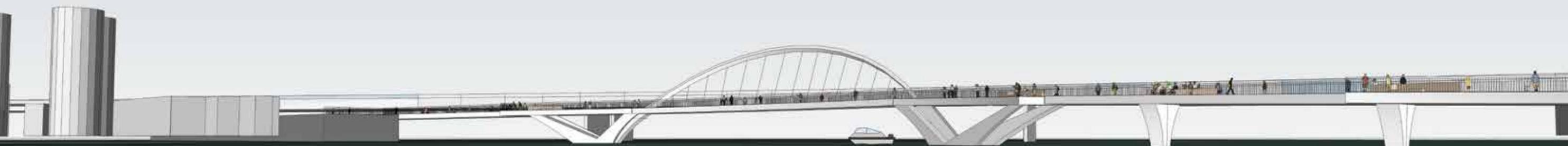
An extra wide span is proposed to enable small boats to pass easily underneath.
